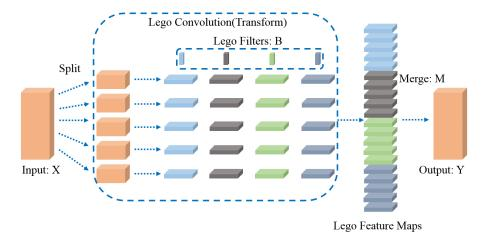
Figure 2. Lego Unit(LU). This figure shows how the three-stage pipeline split-transform-merge operates on input feature maps.  $\mathbf{X}$  is the input feature map, lego filters  $\mathbf{B}$  are convolved with different parts from  $\mathbf{X}$ , which result in intermediate feature maps  $\mathbf{I}$ . Output feature map  $\mathbf{Y}$  is generated by merging according to  $\mathbf{M}$ .
